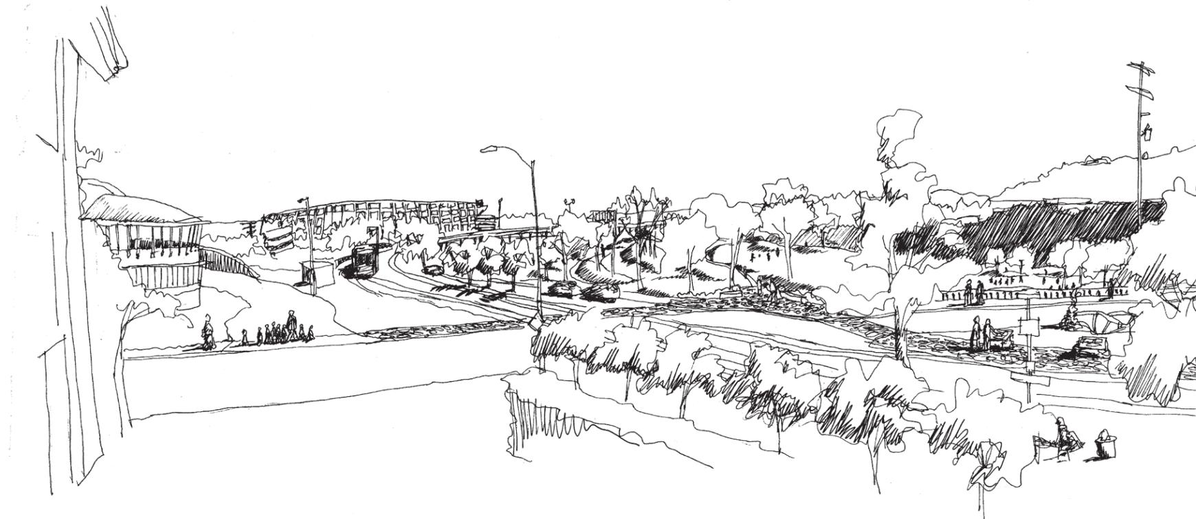
To guide park visitors from the trolley stop, library and street-side parking to the strolling area park entrance, street crossings and sidewalks will be marked by inlaid broken concrete. The broken concrete, which is both recycled and aesthetically interesting, gives reference to the potentially destructive flooding power of the river in this area and allows for increased groundwater infiltration verses conventional paving.
